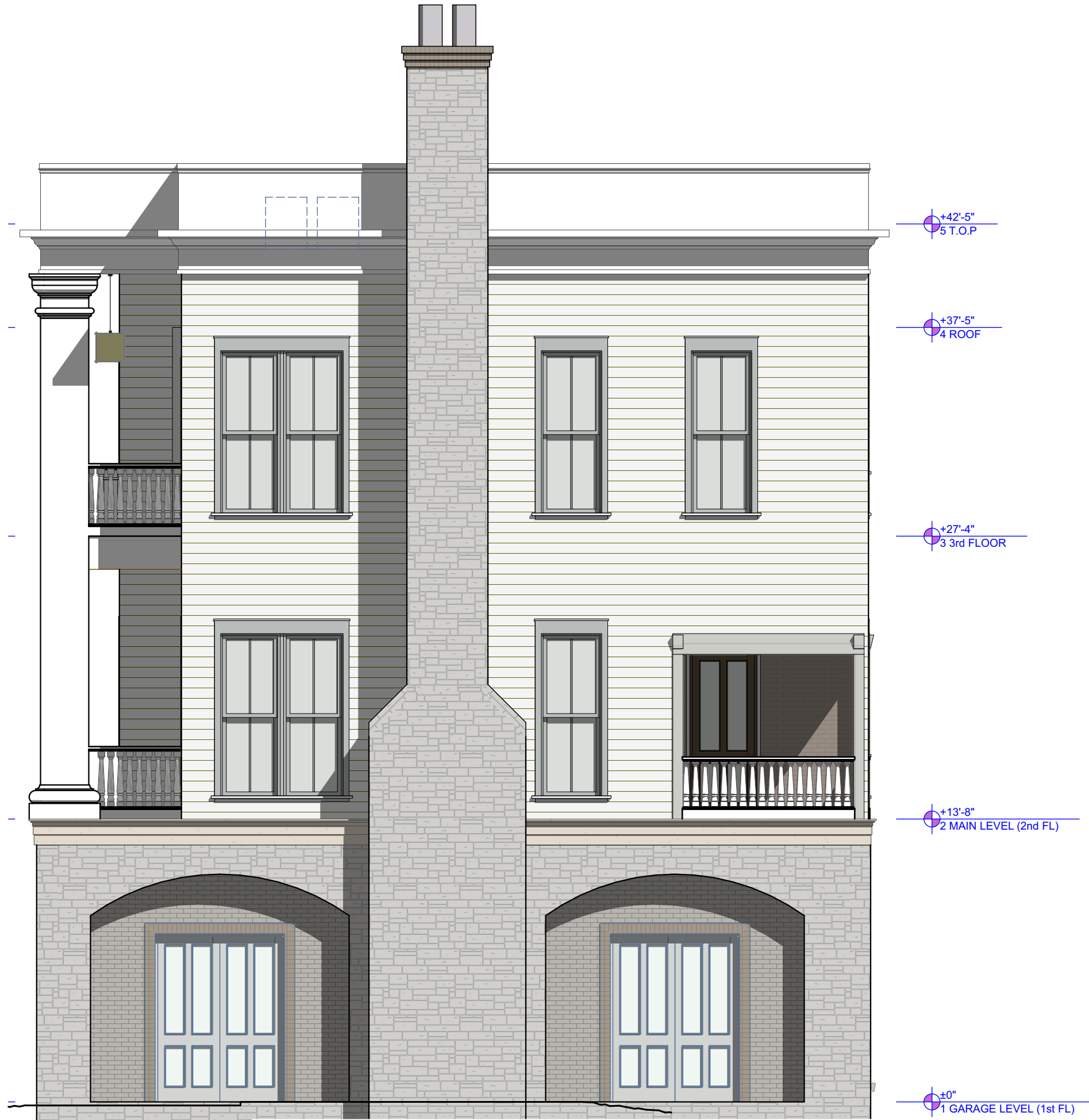
1 REAR Elevation (ALPHA LOOP) SCALE: 3/16" = 1'-0"
