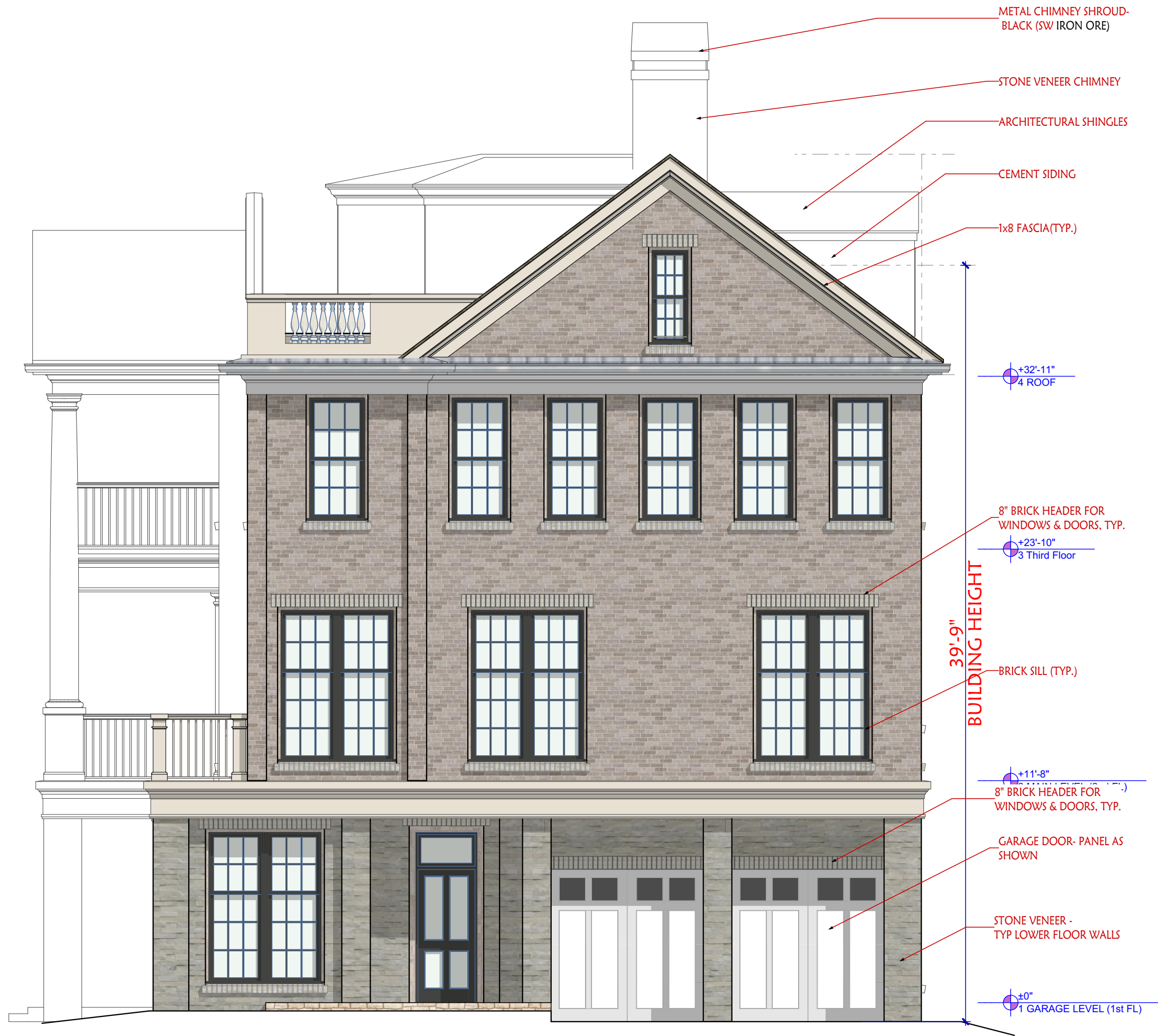
1 FRONT Elevation SCALE: 3/16" = 1'-0"
