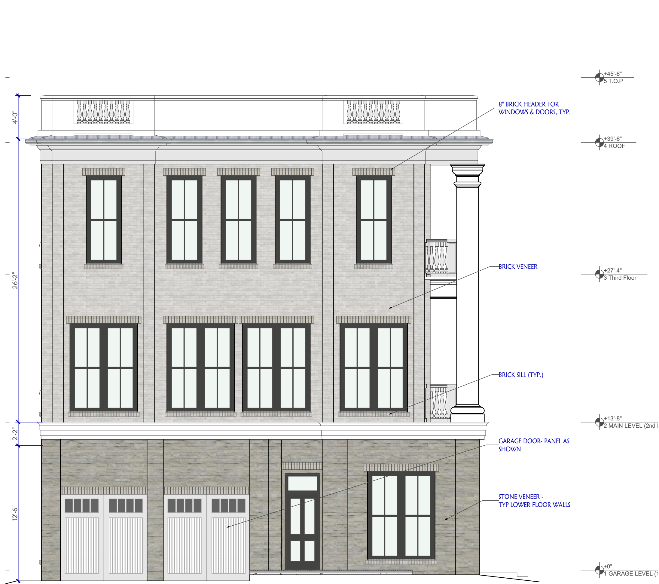
1 FRONT Elevation SCALE: 3/16" = 1'-0"
