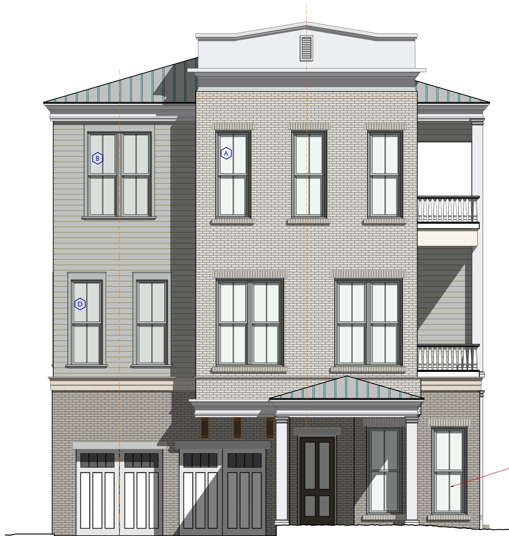
2 FRONT Elevation (MAIN STREET) SCALE: 3/16" = 1'-0"
