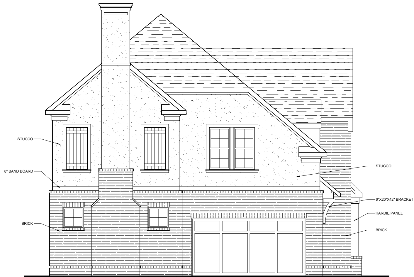
SIDE ELEVATION B - LOT 6 (INTERNAL STREET VIEW)
