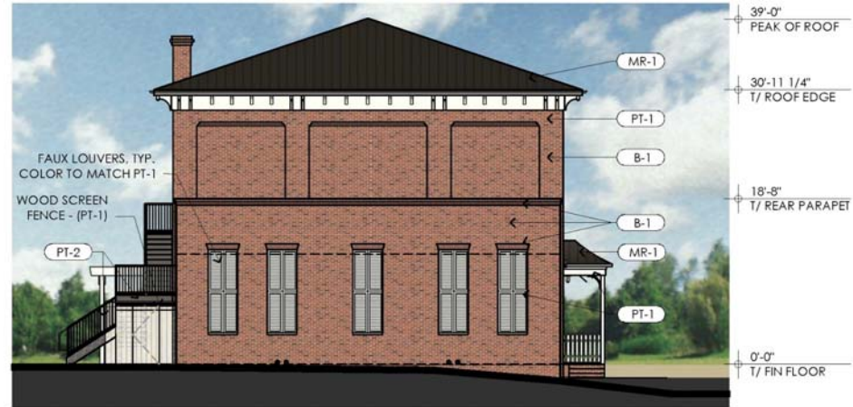
01 EAST ELEVATION A2.2 3/32" = 1'-0"
