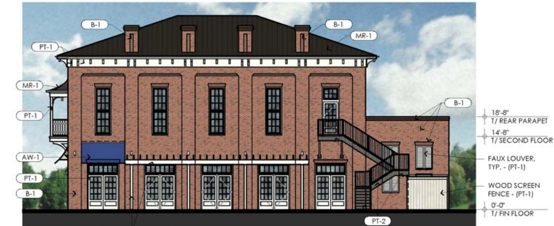
02 SOUTH ELEVATION A2.2 3/32" = 1'-0"
