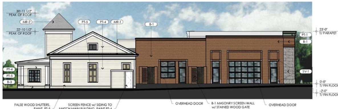
02 NORTH ELEVATION A2.2 3/32" = 1'-0"
