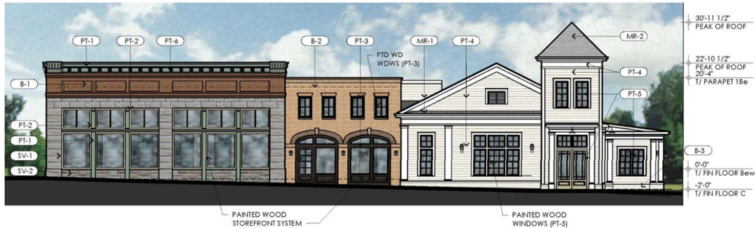
02 SOUTH (N BROAD) ELEVATION A2.1 3/32" = 1'-0"
