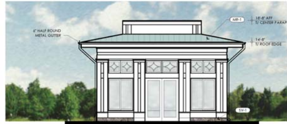
02 WEST (MAIN ST) ELEVATION A2.1 1/8" = 1'-0"
