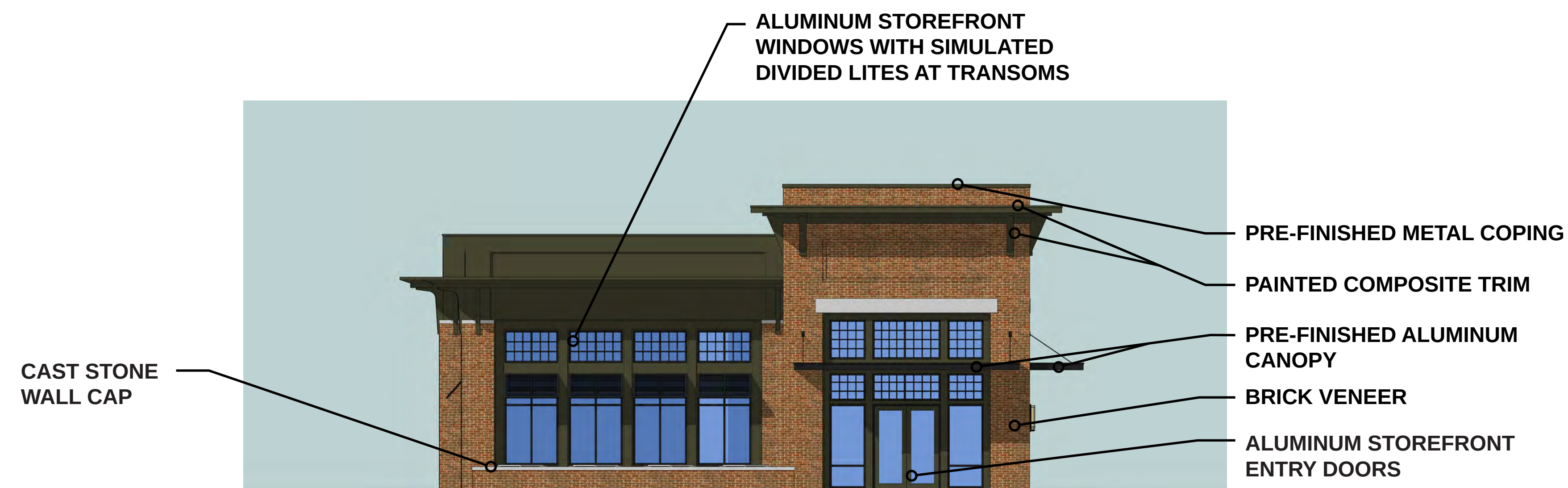
BUILDING 'G' SIDE ELEVATION SCALE: 1/8" = 1'-0"
