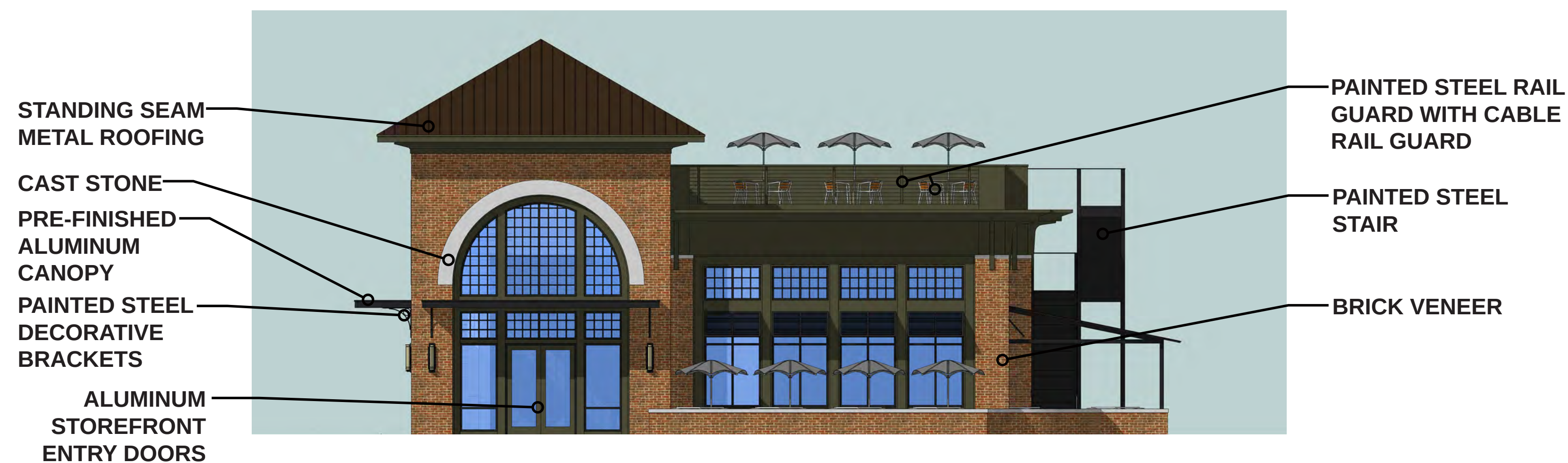
BUILDING 'C' SIDE ELEVATION SCALE: 1/8" = 1'-0"
