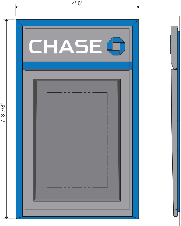
SUR-TTW-U-4-TP THIN PROFILE ATM SURROUND - 33SF SCALE: NTS
