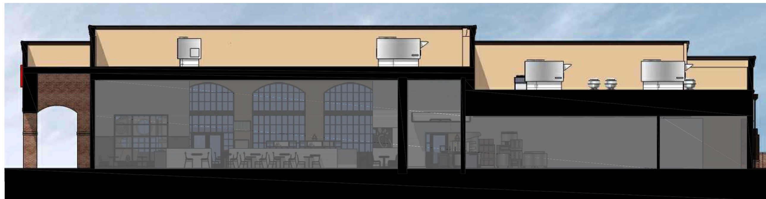
Section Showing Rooftop Equipment 3/32" = 1'-0" Scale
