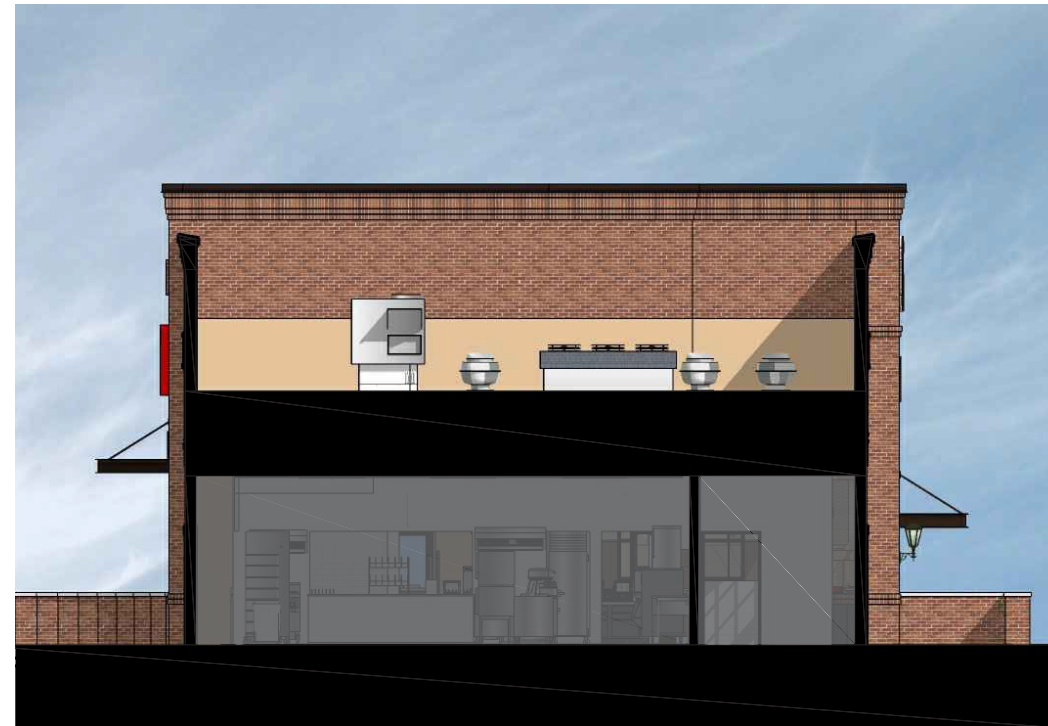
Section Showing Rooftop Equipment - High Roof 3/32" = 1'-0" Scale
