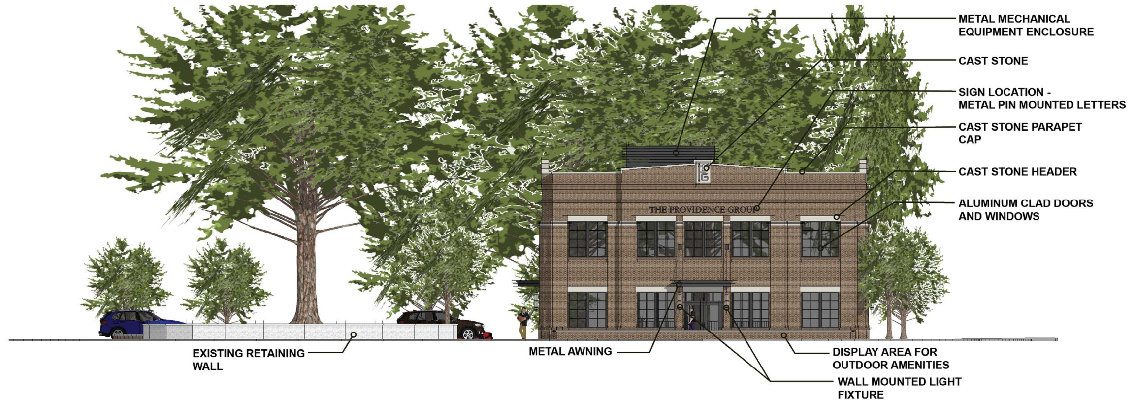
EAST ELEVATION - ENTRY CIRCLE
