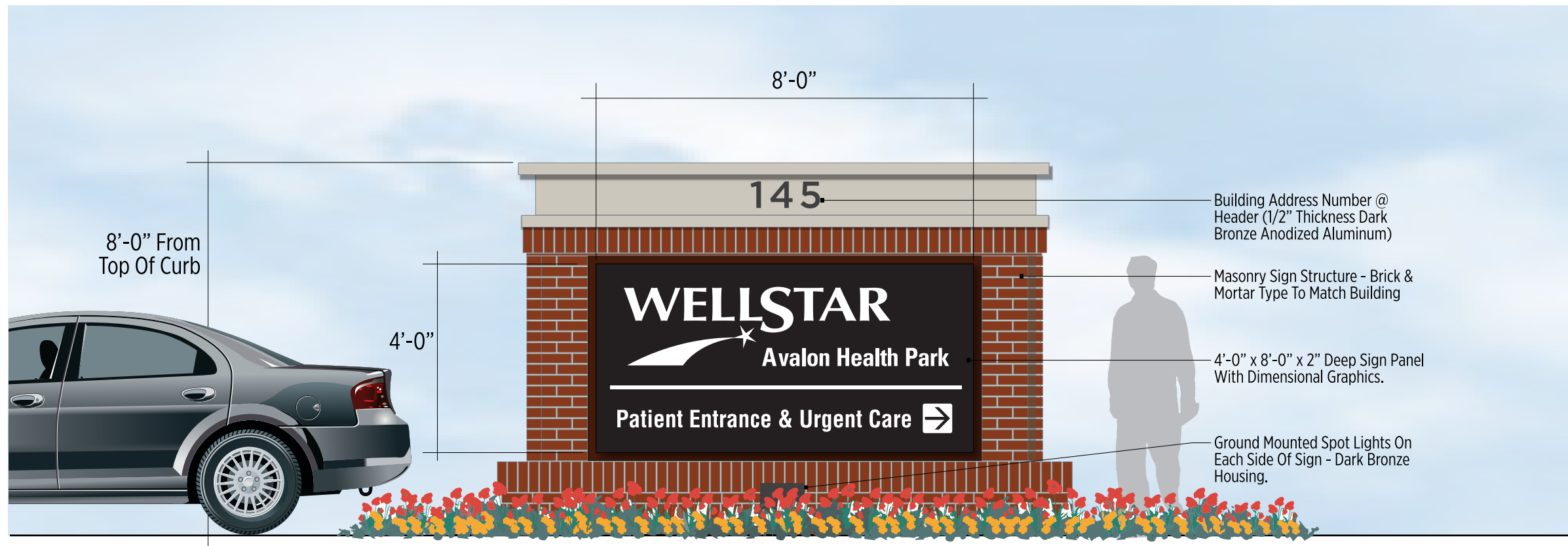
A Proposed Sign Elevation (Opposite Side Is Similar) Scale: 3/8" = 1'-0"
