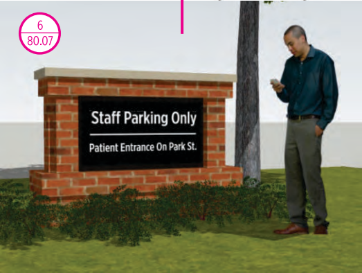
Monument Sign at Staff Entry - Ground Lighted
