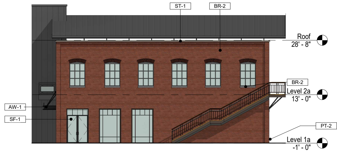
BUILDING 3 SOUTH ELEVATION
