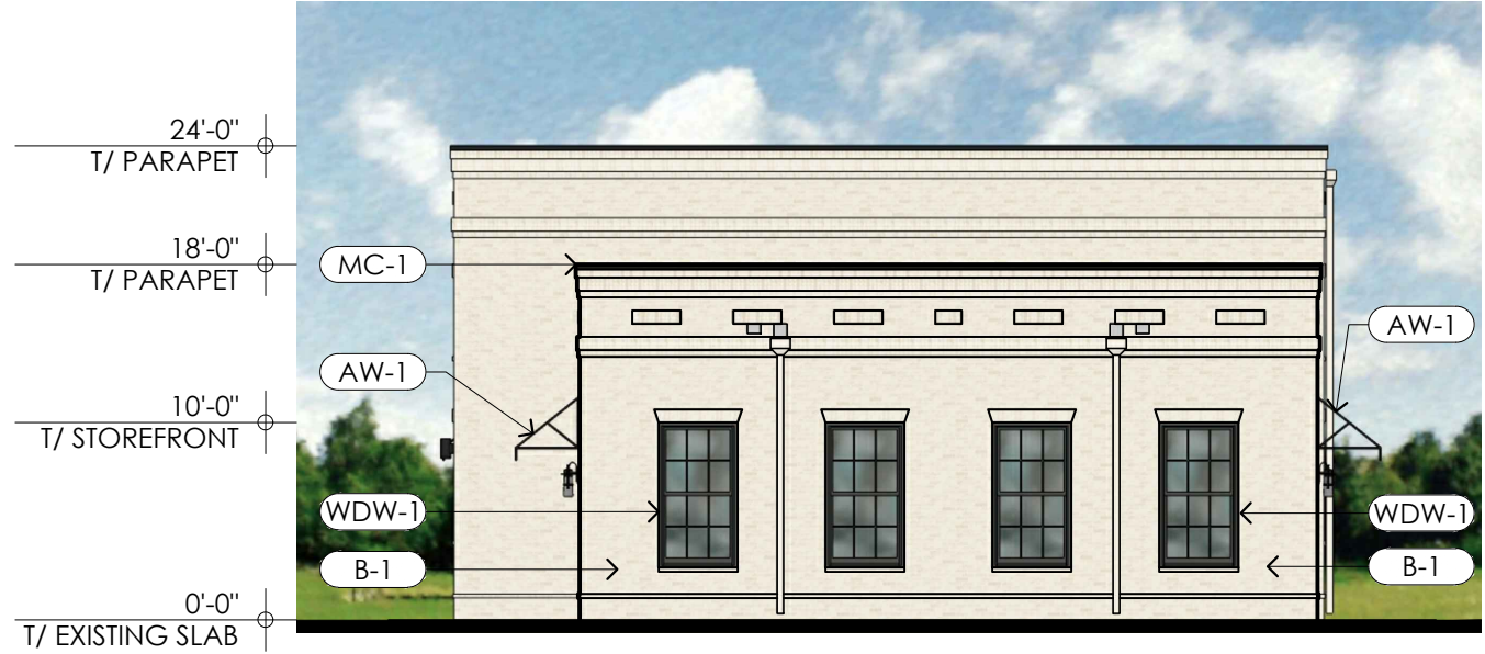
02 EAST ELEVATION (ENTRY DRIVE) A2.1 SCALE: 3/32" = 1'-0"
