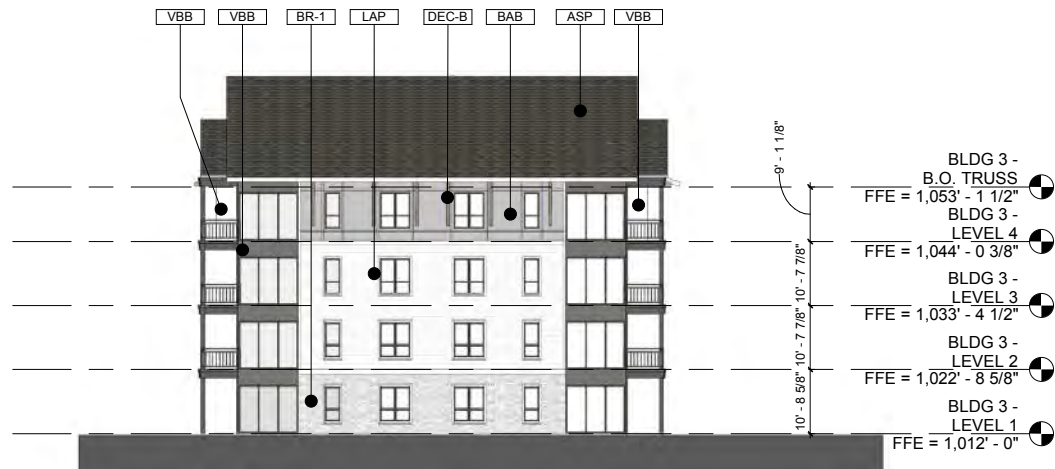
3 BLDG 3 - OVERALL EAST ELEVATION 1/16" = 1'-0"
