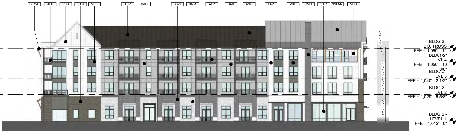
3 BLDG 2 - OVERALL WEST ELEVATION 1/16" = 1'-0"
