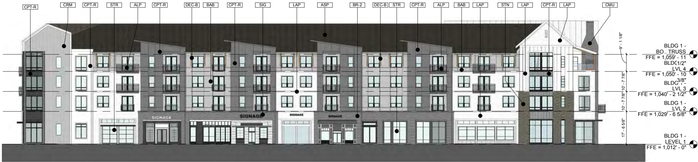
2 BLDG 1 - OVERALL SOUTH ELEVATION 1/16" = 1'-0"
