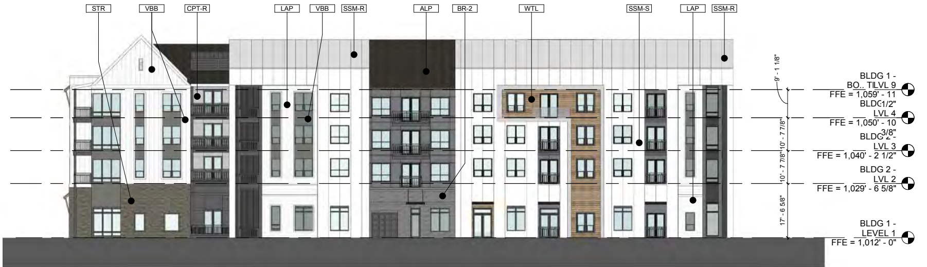
3 BLDG 1 - OVERALL WEST ELEVATION 1/16" = 1'-0"
