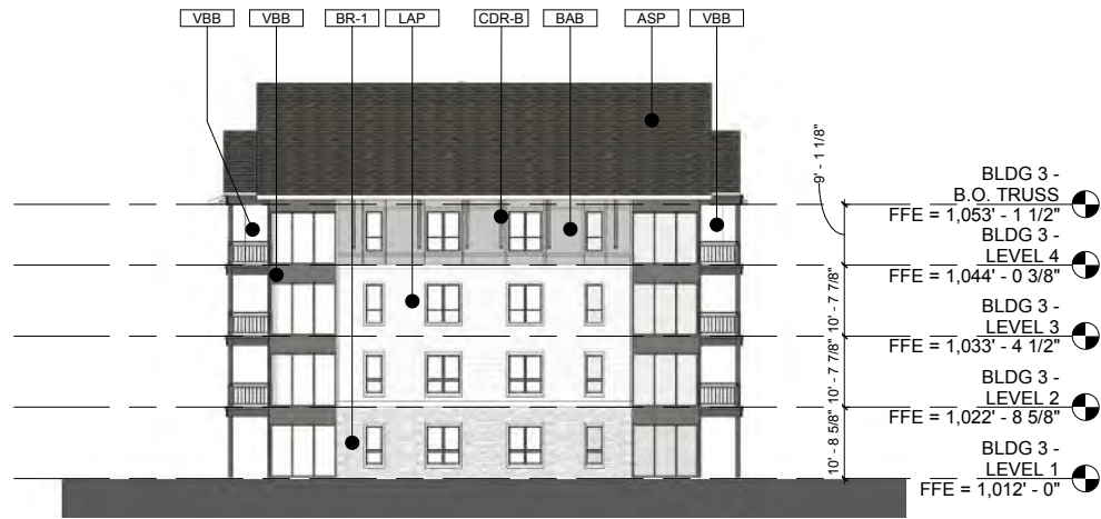
4 BLDG 3 - OVERALL WEST ELEVATION 1/16" = 1'-0"
