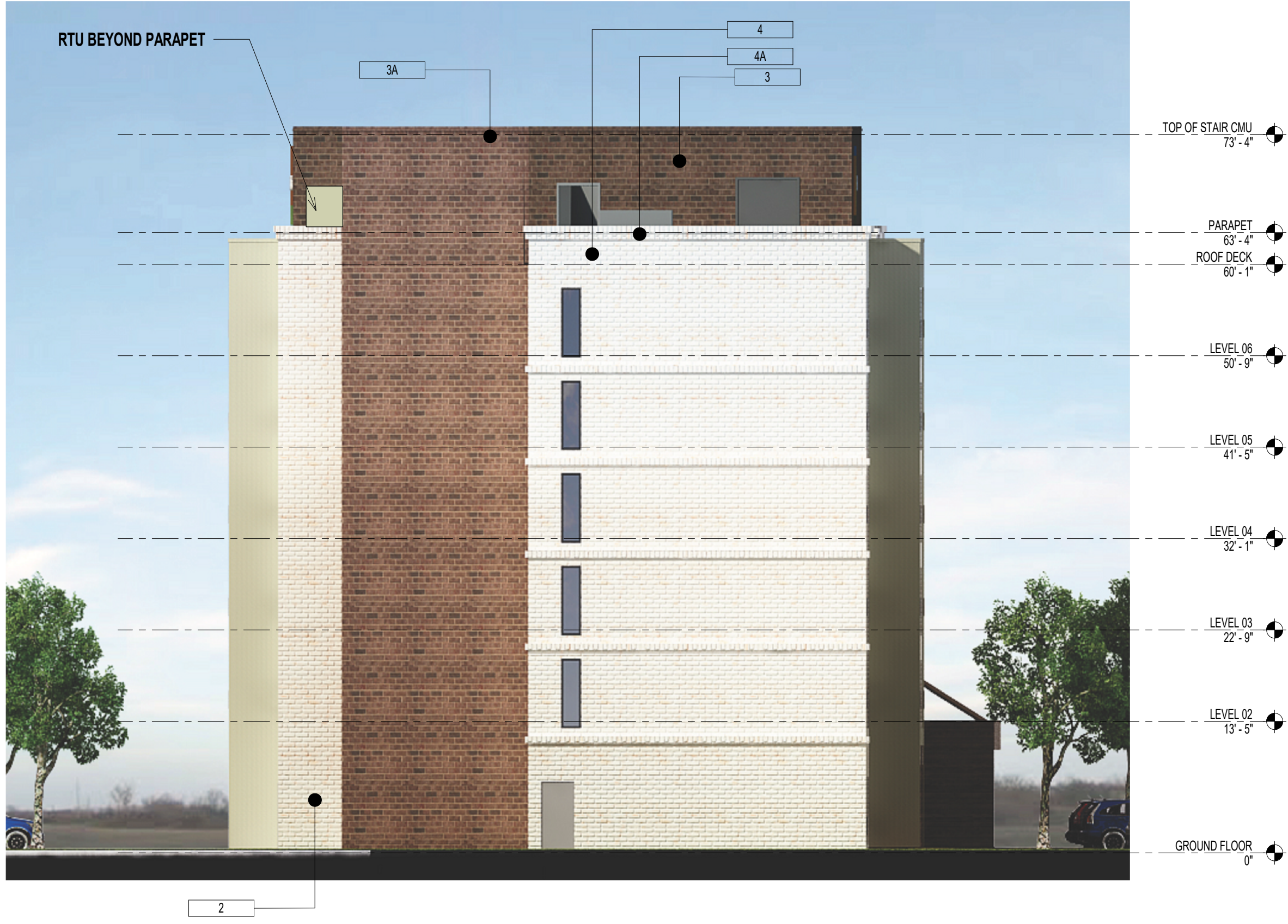
3 WEST ELEVATION- SCALE: 3/32" = 1'-0"
