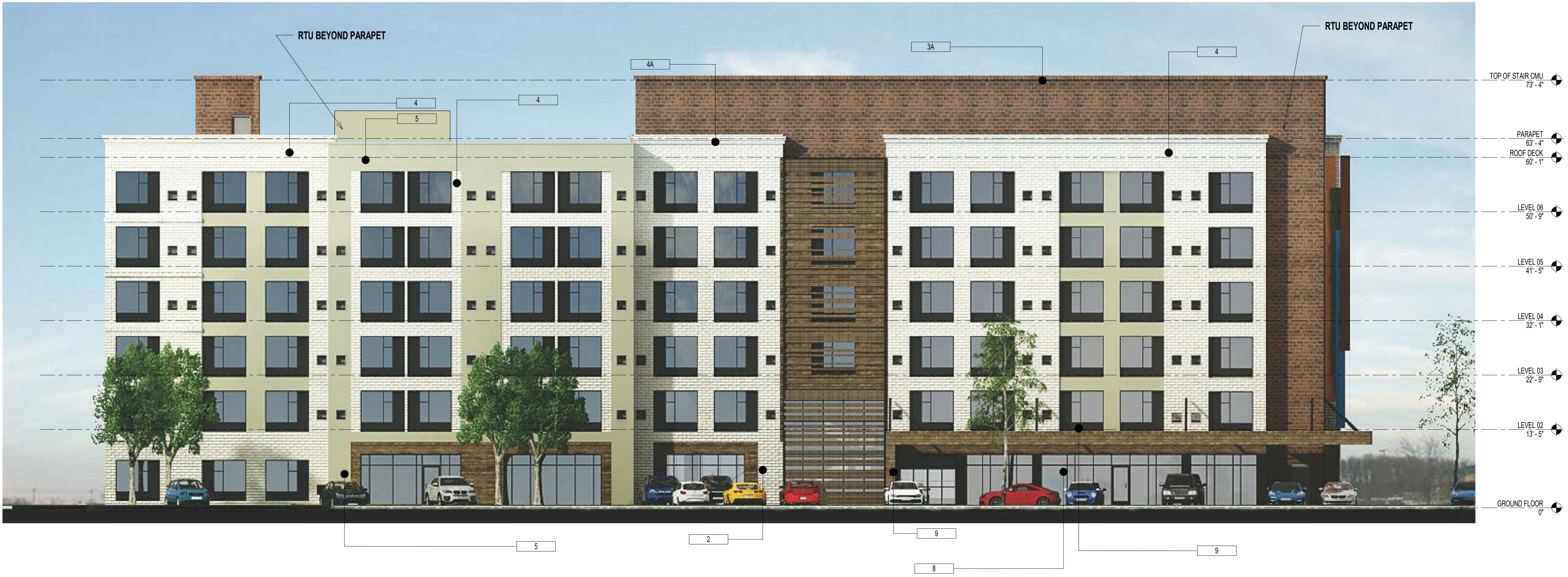
1 SOUTH ELEVATION- SCALE: 3/32" = 1'-0"
