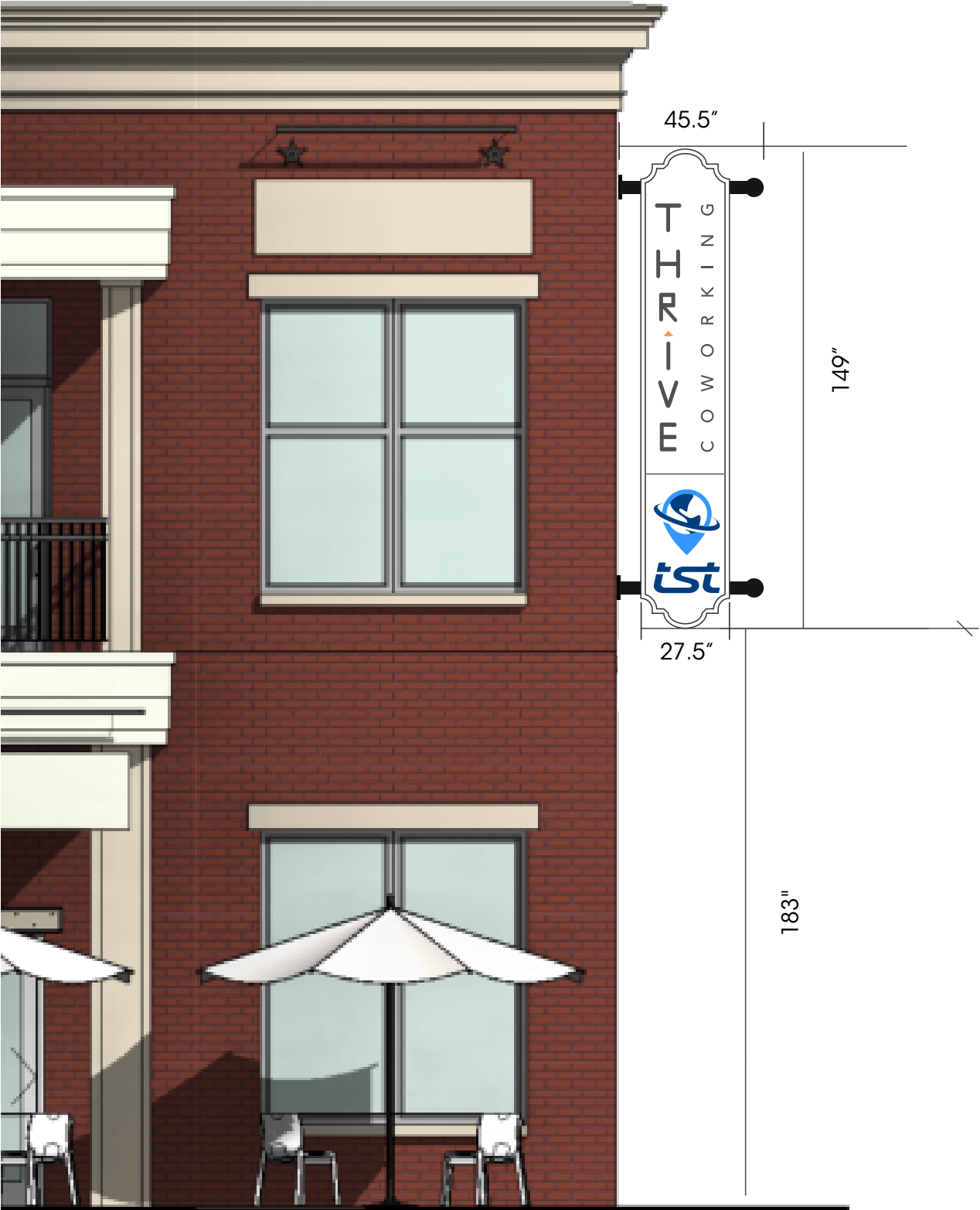
Description: Projecting Non-Illuminated Aluminum Cabinet with 1" Thick Pin Mounted Acrylic Letters. Double Sided. "COWORKING" - .5" THICK ARYLIC
