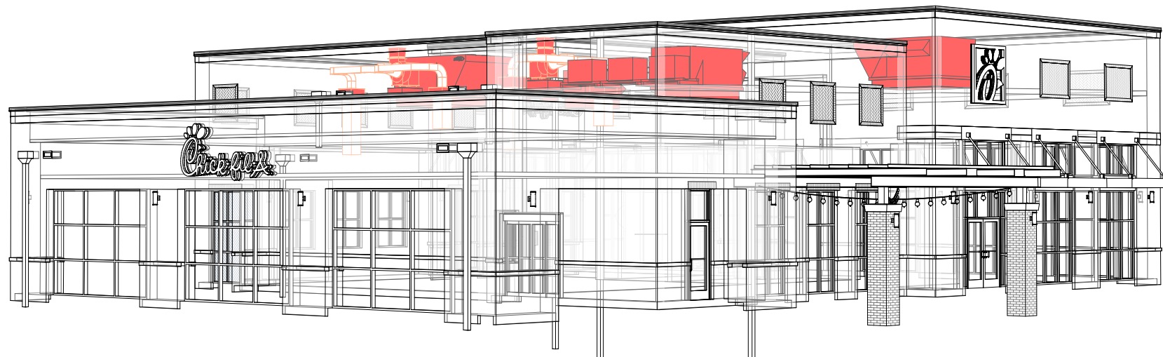
ROOF EQUIPMENT SCREENING PERSPECTIVE 3
