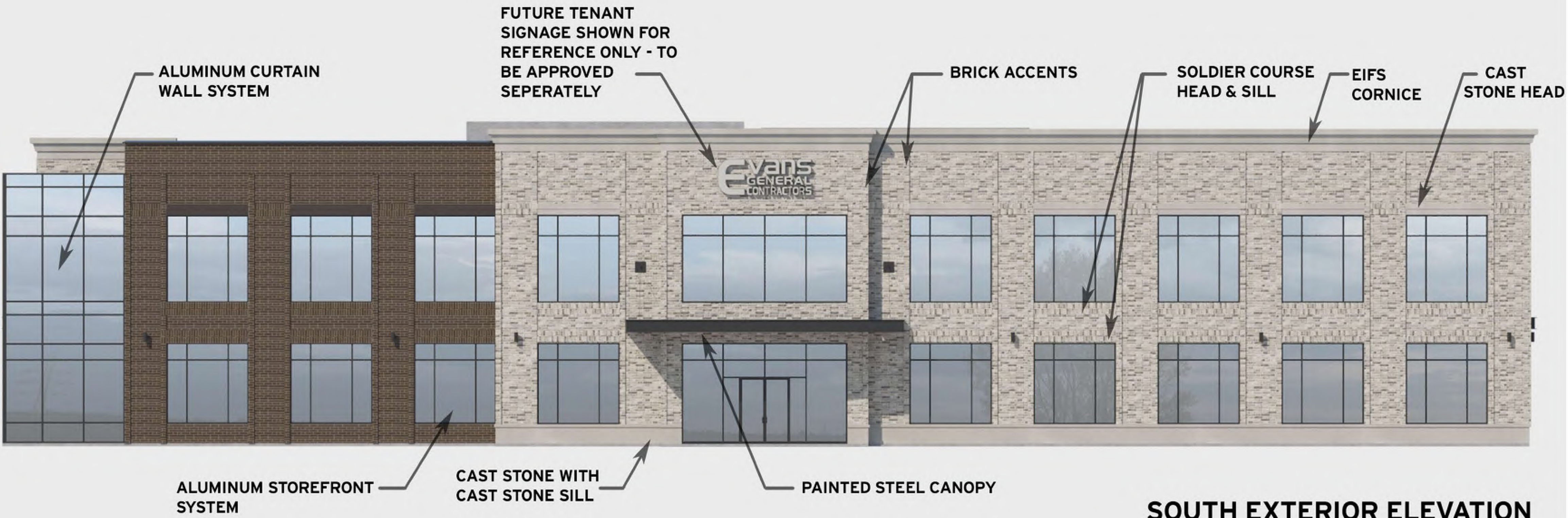
SOUTH EXTERIOR ELEVATION
