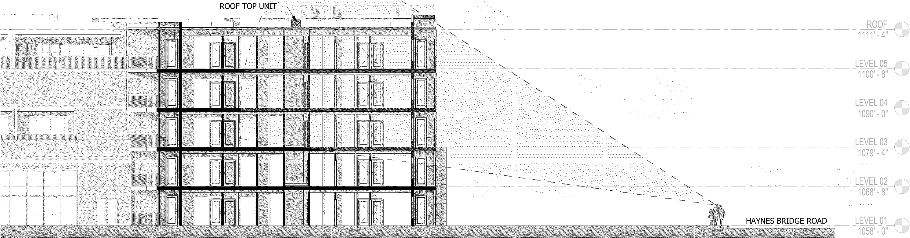
SITE LINE STUDY - EAST ELEVATION
