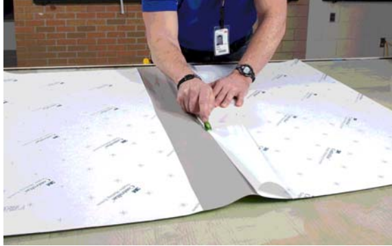
FIGURE 13 Cutting Out Section of Liner for Self Hinge
