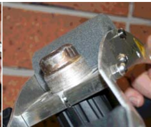
FIGURE 23 Positioning Heat Gun Nozzle in Heat Gun Holder
