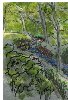
Channel with stabilized banks and buffer vegetation
