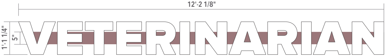
1 CUSTOM ILLUMINATED CHANNEL LETTERS - RACEWAY 13.4 SF SCALE: 1/2" = 1'-0"
