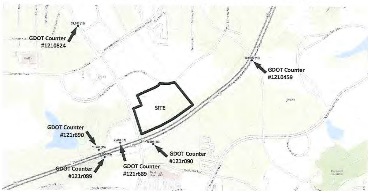
Figure 2: Traffic Counter Locations
