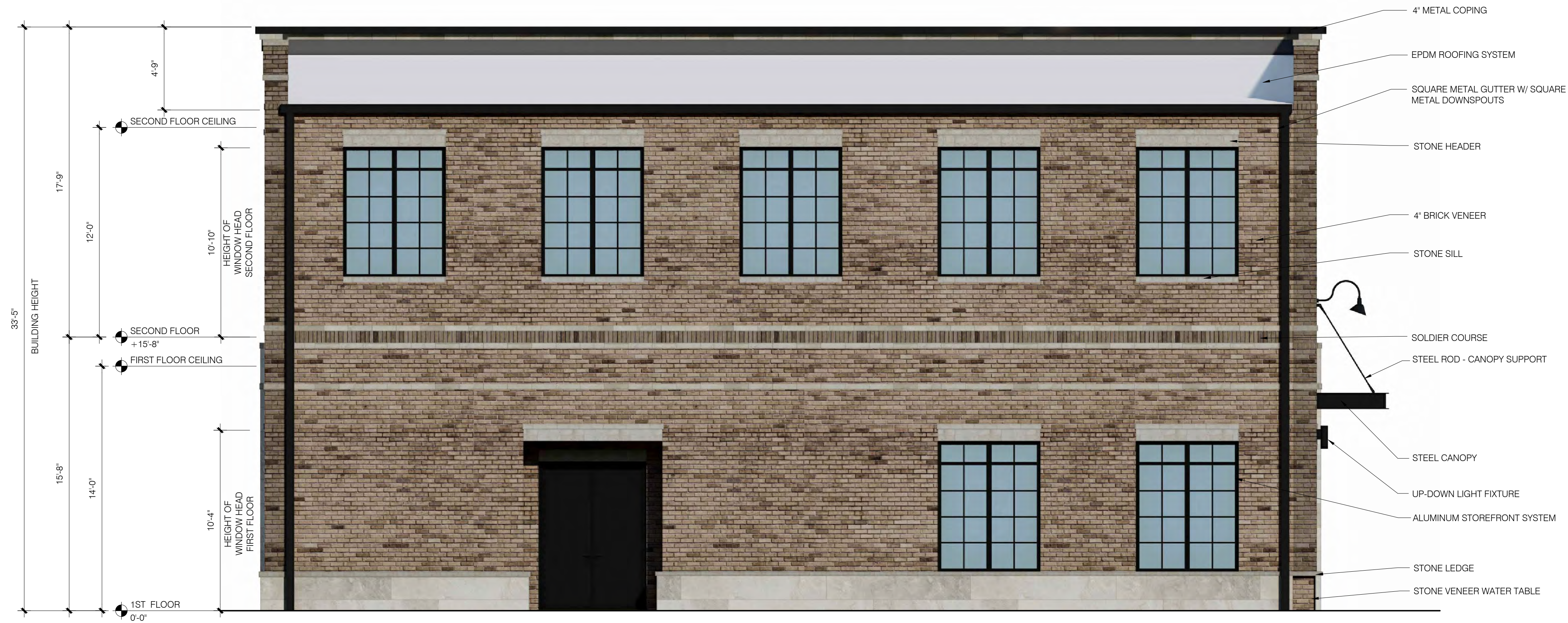
1 rear elevation A4.2 SCALE: 1/4" = 1'-0"
